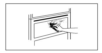
DO NOT ATTEMPT TO REMOVE ANY OF THE CONTROL KNOBS FROM THE PANEL AS THIS MAY CAUSE DAMAGE AND IS A SAFETY HAZARD.
